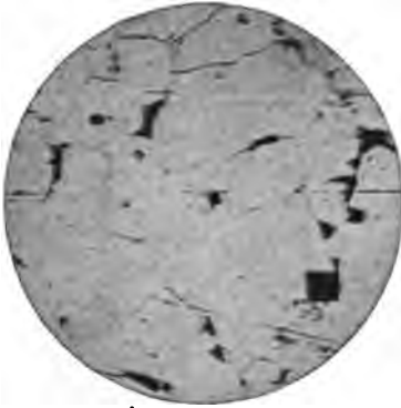
Fig. 9. Ferrite and Pearlite; Carbon, 0.05 Per Cent
